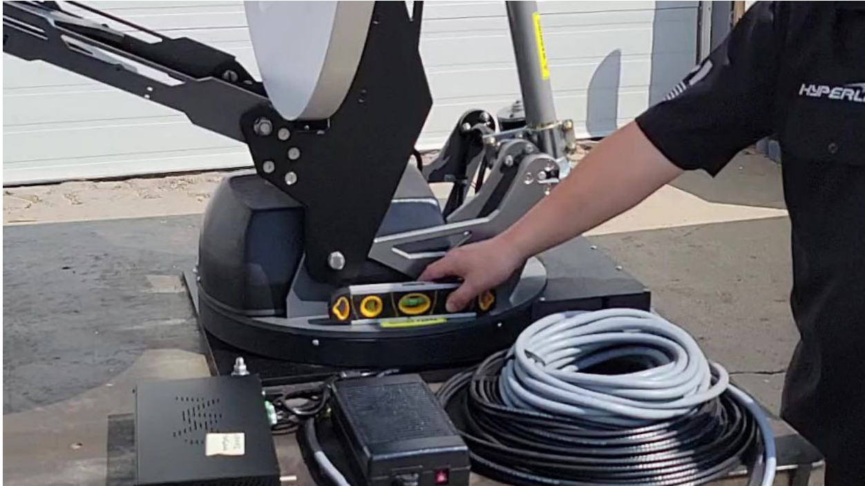
Level the base front to back
